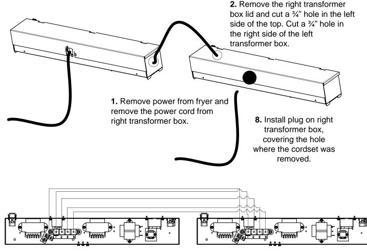
**3.** Remove the lid from each box and connect the provided wire harness to the terminal block in the left transformer box. Follow the color code established by the power cord.
